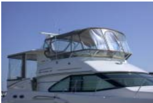
Bridge and aft deck enclosure
